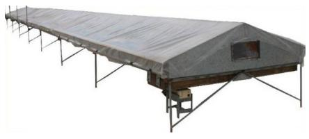
The MCSTD is designed to utilize solar heat in drying while keeping the commodities clean. Adapted from the design of Hohenheim University in Germany, it was modified to suit the needs of local farmers engaged in processing.
